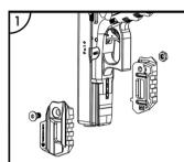
PLACE THE TWO HALVES OF THE RAIL IN POSITION ON THE GUN. SECURE TOGETHER WITH THE SUPPLIED HARDWARE.
